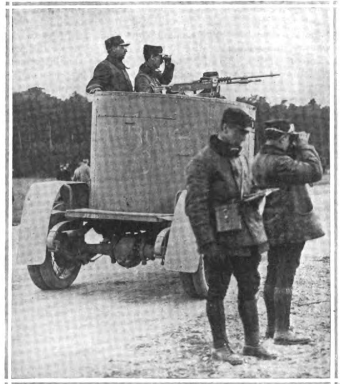
Above—One of a corps of Belgian armored cars reconnoitering on a road in the north of France. Note under-slung rear springs and dual tires
